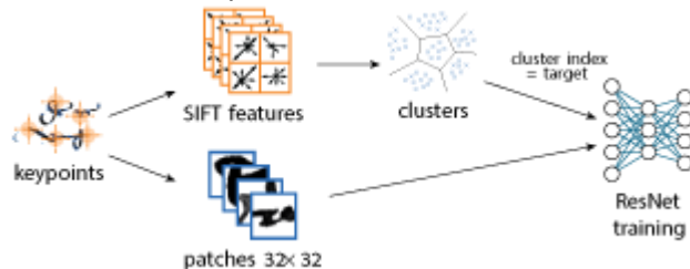
Figure 4 Workflow of the [6] The patches are extracted on the location of the keypoints. The CNN is told to classify these patches according to a clustering of their descriptors.
