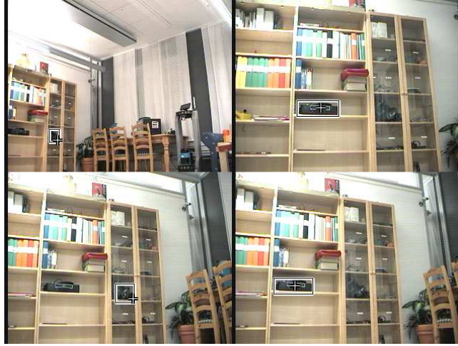
Fig. 6. Two matches of ROIs (rectangles) and Harris-Laplace points (crosses) between a current frame (top) and a scene from the database (bottom).
