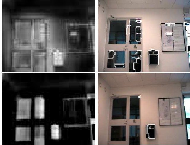
Fig. 3. Saliency maps (top, left: S_{bu} , bottom, left: S_{td} ) and MSRs in a loop closing example: Top: scene at beginning of sequence (all MSRs shown). Bottom: revisited scene, 592 frames later, searching for the black waste bin with top-down attention (only most salient MSR shown).
