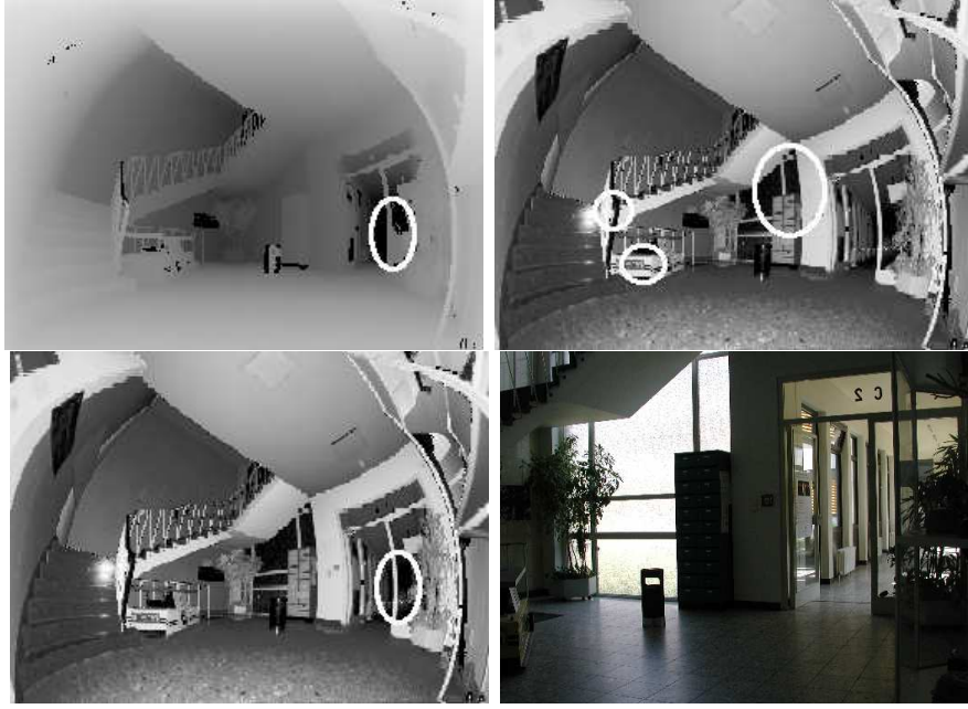
Fig. 8. The foci in laser data show some advantages of the depth mode. In reading order: depth image, reflection image, combined image, camera image. The open door is salient only in the range data.
