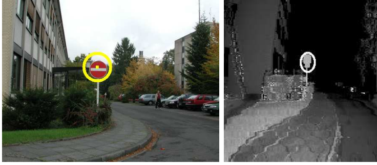
Fig. 11. Foci showing the same region in camera and in laser data. Left: a camera image with a focus on a red traffic sign generated by the NVT. Right: a laser image, combined from depth and reflection data, with a focus generated by BILAS.
