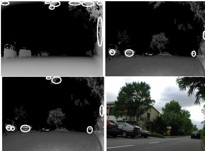
Fig. 10. The foci in laser data show some advantages of the reflection mode. In reading order: depth image, reflection image, combined image, camera image. All of the four cars are among the first six focus regions in the reflection data.
