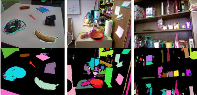
Fig. 11. Top: some examples of our object discovery method on real-world office scenes. Each colored contour shows one detected object hypothesis. Bottom: separately displayed object hypotheses of the above images.
