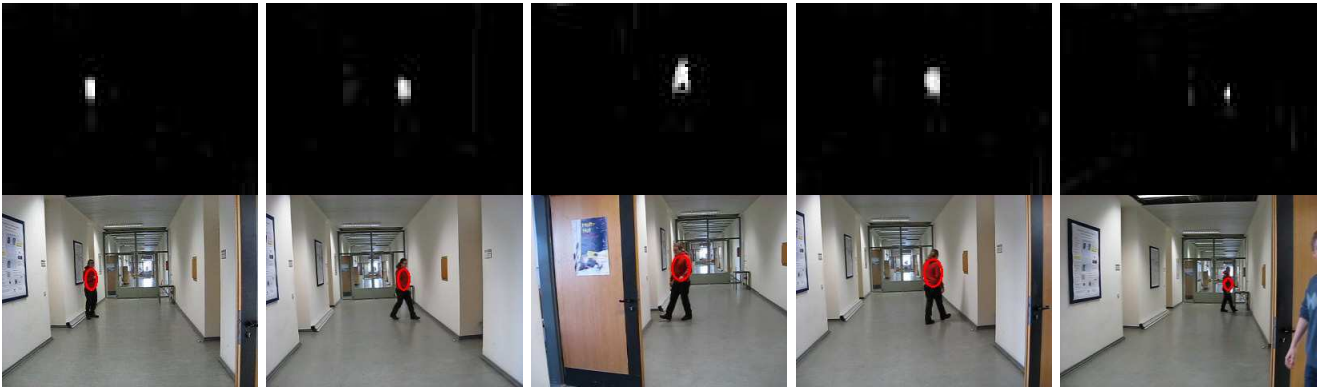
Fig. 4. Person tracking with cognitive data association. Top: the top-down saliency map. Bottom: the corresponding input image with the resulting FOA (focus of attention) displayed as red ellipse. The person is tracked successfully in all frames.
