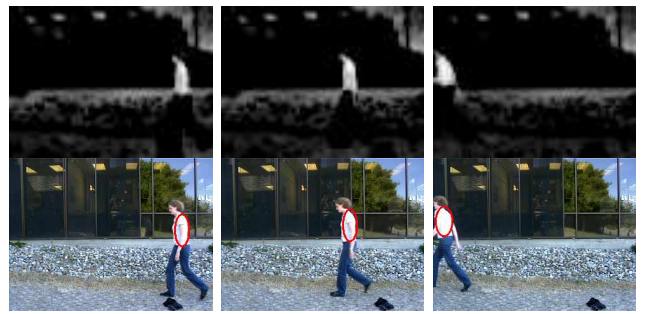
Fig. 3. Person tracking with cognitive data association on a standard test sequence 1 [37]. Top: the top-down saliency map. Bottom: the corresponding input image with the resulting FOA (focus of attention) displayed as red ellipse.
