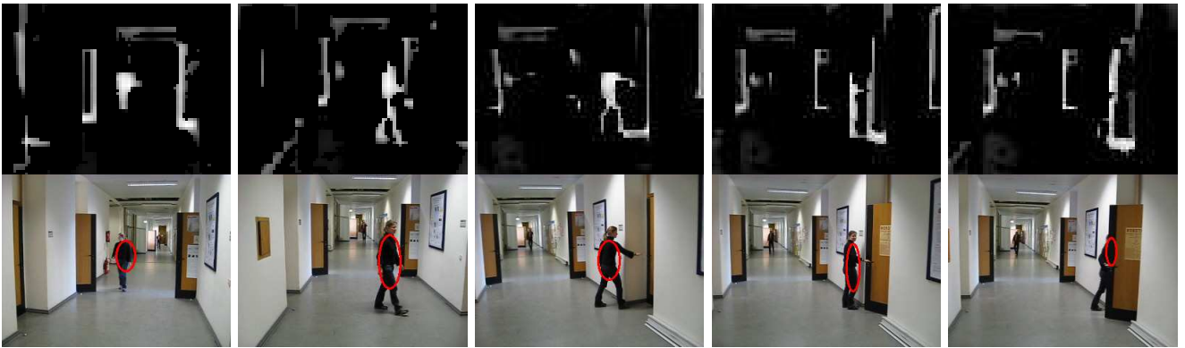
Fig. 5. Person tracking with cognitive data association. Top: the top-down saliency map. Bottom: the corresponding input image with the resulting FOA (focus of attention) displayed as red ellipse. The person is tracked successfully, until it goes through the door on the right. Here, the system confuses the person with the black stripe of the door.
