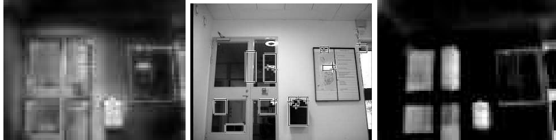
Fig. 2. Left: bottom-up saliency map. Middle: attentional ROIs (rectangles) and Harris corners (crosses). Right: top-down saliency map for target “wastebin” (black box).
