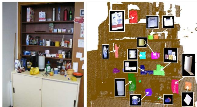
Fig. 6: Discovered objects in one of our sequences. Left: original scene. Right: 3D map with 19 discovered objects by the end of the sequence. The rectangles show the automatically obtained 2D object candidates from the color processing stream. Fig. from [9].
