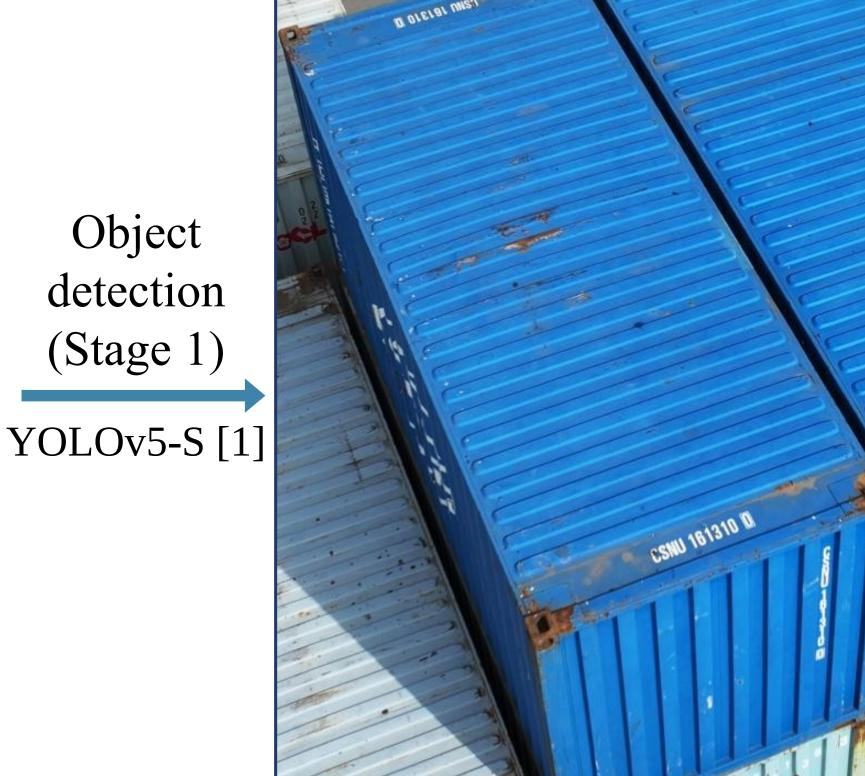
Text Detection (Stage 2) DBNet++ [2] CSNU 161310 0 Text Recognition TrOCR [3] (Stage 3)
