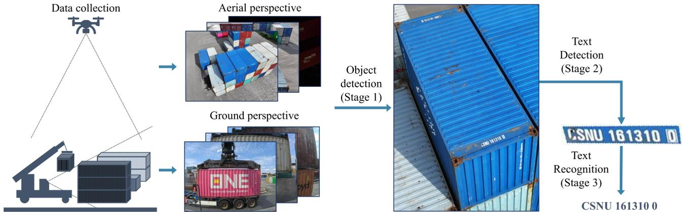
**Fig. 1:** This study presents a framework for inland ports that uses unmanned aerial vehicle (UAV)-based imaging, and reach stacker sensor data including a camera to monitor port operations. A three-stage identification pipeline detects transportation units (TUs) as the first stage, then markings of detected TUs such as ISO6436 compliant ID codes are detected as the second stage. Finally, a text recognition model extracts their IDs.
