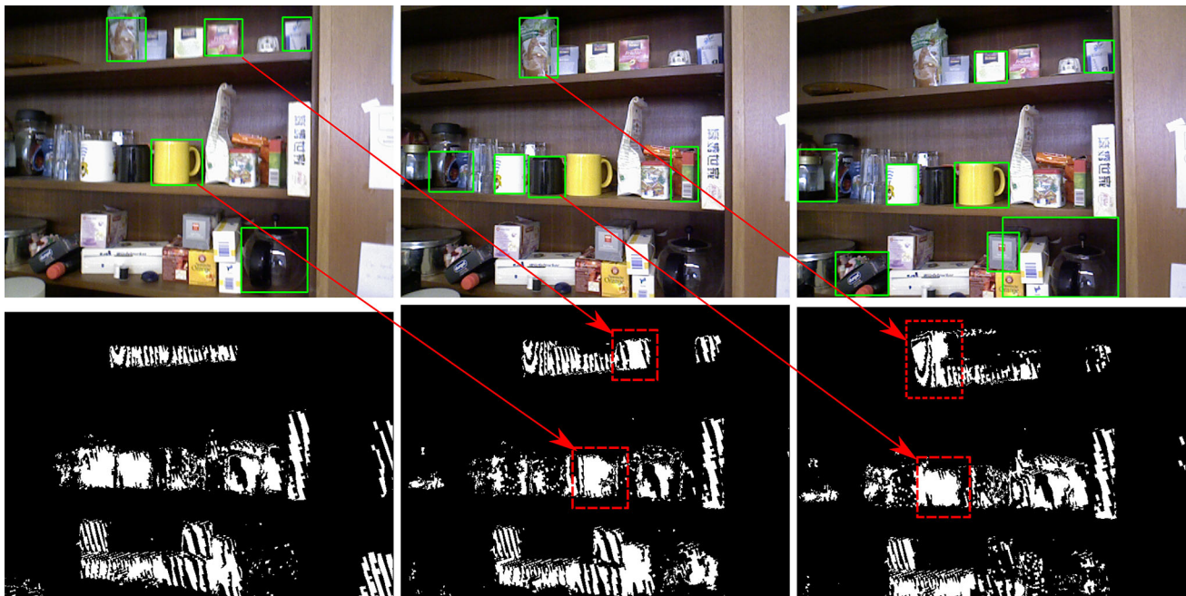
Fig. 12 Illustration of the IOR experiment: on top some frames from the Coffee Machine Sequence; the green bounding boxes show the candidates that successfully matched an object. The bottom row
