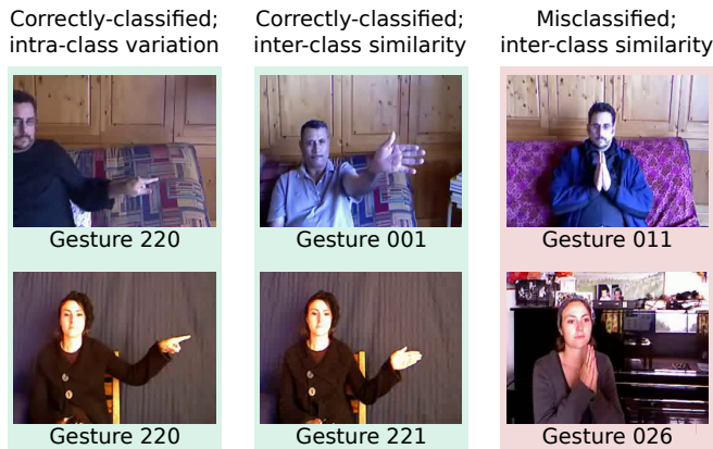
Fig. 4. Left and Middle: Correctly-classified gestures. Right: Gesture 011 mostly misclassified as Gesture 026.
