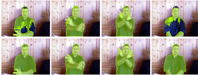
Fig. 7: Comparison of segmentations of the signer’s body with SAM (upper row) and SAM 2 (lower row) in SegSLR on four frames of a video from the ChaLearn249 IsoGD test dataset.
