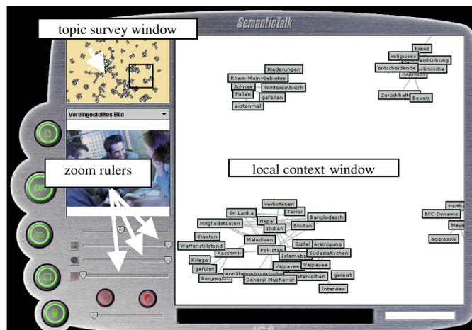
**Figure 1:** The *SemanticTalk* user interface. The local context window is a zoomed variant of the topic survey window and can be changed with the three zoom rulers. Other controls: New, Load, Save, Exit, Microphone on/off, Freeze graph, Brainstorming / Red thread Switch, Input text bar and scrolling
