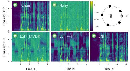
→ Joint non-linear spatial-spectral filter is a more powerful processing model
