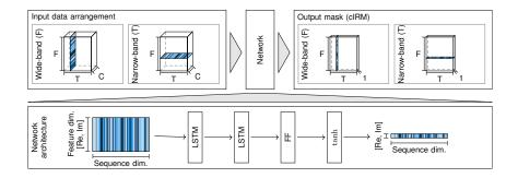
Network structure that allows to easily control the integration of different sources of information
