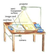
Figure 1. Setup of the Tangible Interface.
