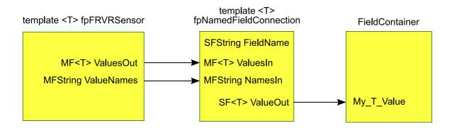
Figure 3: The class descriptions of MultiField reflection system of FRVR-AVANGO. The fpFRVRSensor and fpNamedFieldConnection template classes allow access to the run-time defined "Fields" as if they were normal Fields through their tags.
