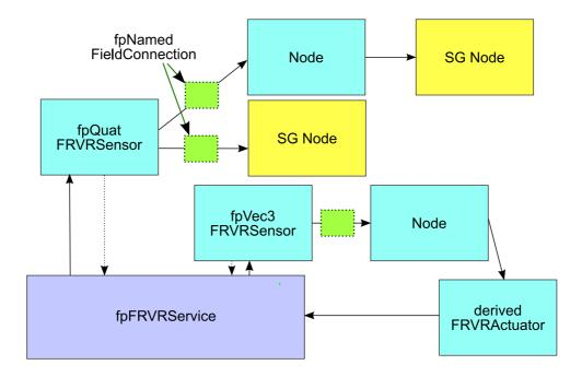
Figure 4: The flow of data through the extended FRVR-AVANGO system. Incorporating the fpNamedFieldConnection objects, removes the need for extending C++ classes to access FRVR values.
