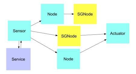
Figure 1: A demonstative data-flow in the AVANGO system. Data flows from the sensors, through various nodes to actuators and SG derived nodes.
