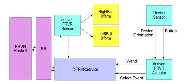
Figure 2: This figure shows the flow of information in the FRVR AVANGO coupling, on hand an implementation of a Newton's Cradle. The derived Sensor and Actuator classes are extended with Fields to deliver/receive the values from/to the FRVR system.
