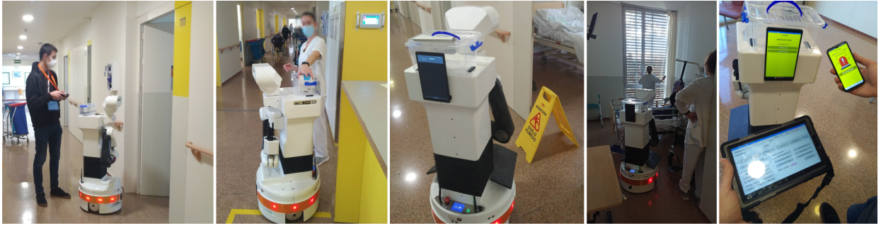
Fig. 5. In-situ teleoperating and testing the robot in the geriatric unit. From left to right: researcher teleoperating the robot; nurse interacting with the robot in a delivery task; robot detecting obstacles in its path (common in the given use case); robot delivering an item to a patient in a room; and prototype applications used in different devices to both, interact with and teleoperate the robot.
